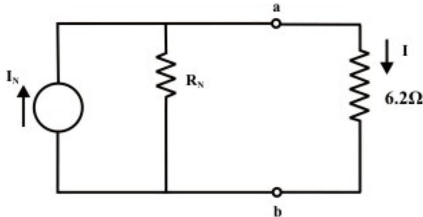
Fig. 8.12(d): Norton's equivalent circuit of original circuit
